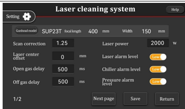
Figure 3-10 Setting interface of cleaning system
