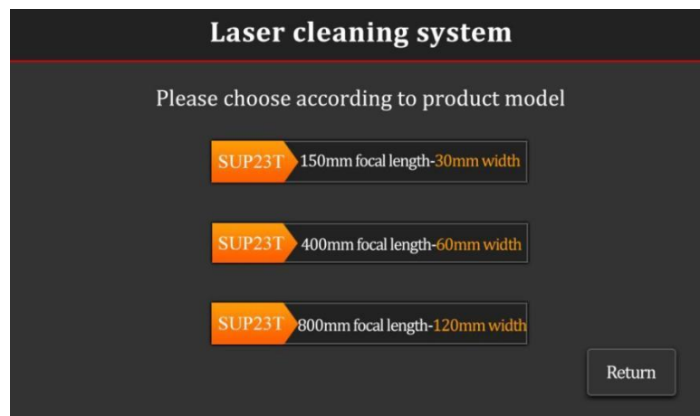
Figure 3-12 Focus lens selection interface
