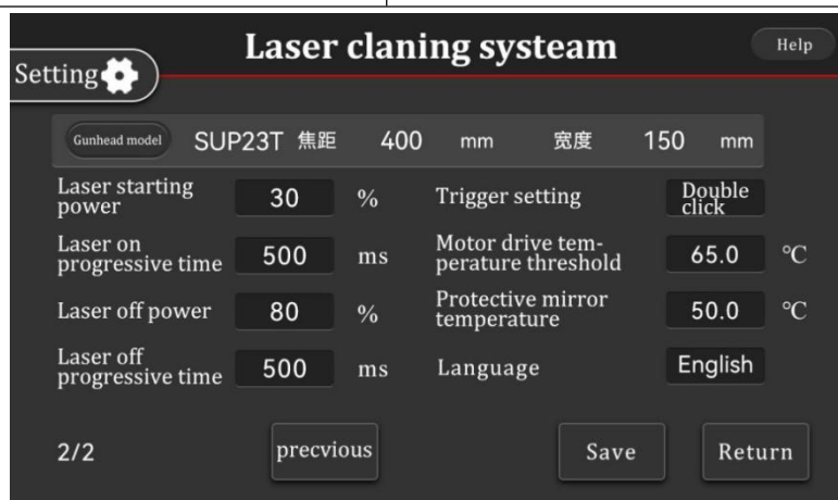
Figure 3-11 Setting interface of cleaning system
